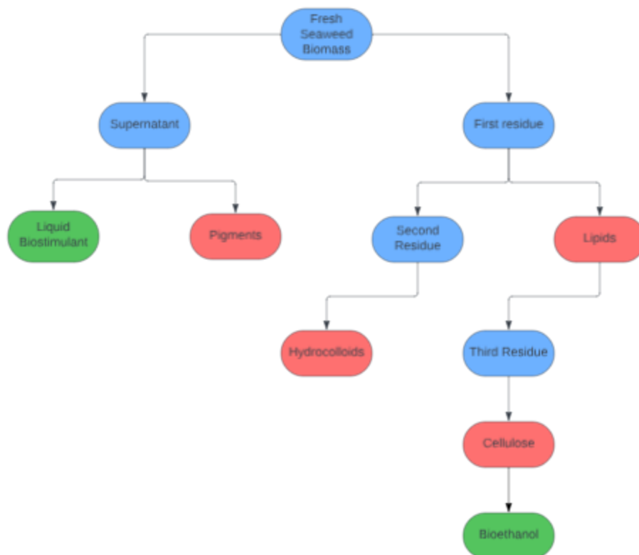
Figure 12: Patented process which produces a liquid biostimulant, natural pigments, hydrocolloids, lipids, and cellulose (Reddy et al., 2018). Blue boxes indicate intermediary steps, green boxes indicate products with GHG mitigating potential, and red boxes indicate other extracted compounds and final products.
