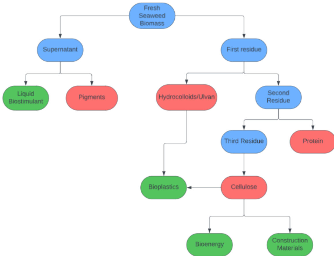
Figure 14: Proposed concept for the extraction of a liquid biostimulant, pigments, hydrocolloids/ulvan, protein, and cellulose from green or red seaweed. Blue boxes indicate intermediary steps. Green boxes indicate final products with GHG mitigating potential. Red boxes indicate other extracted compounds. The production of bioplastics, bioenergy, and construction materials are not detailed in this concept, but are suitable uses for hydrocolloids/ulvan and cellulose.
